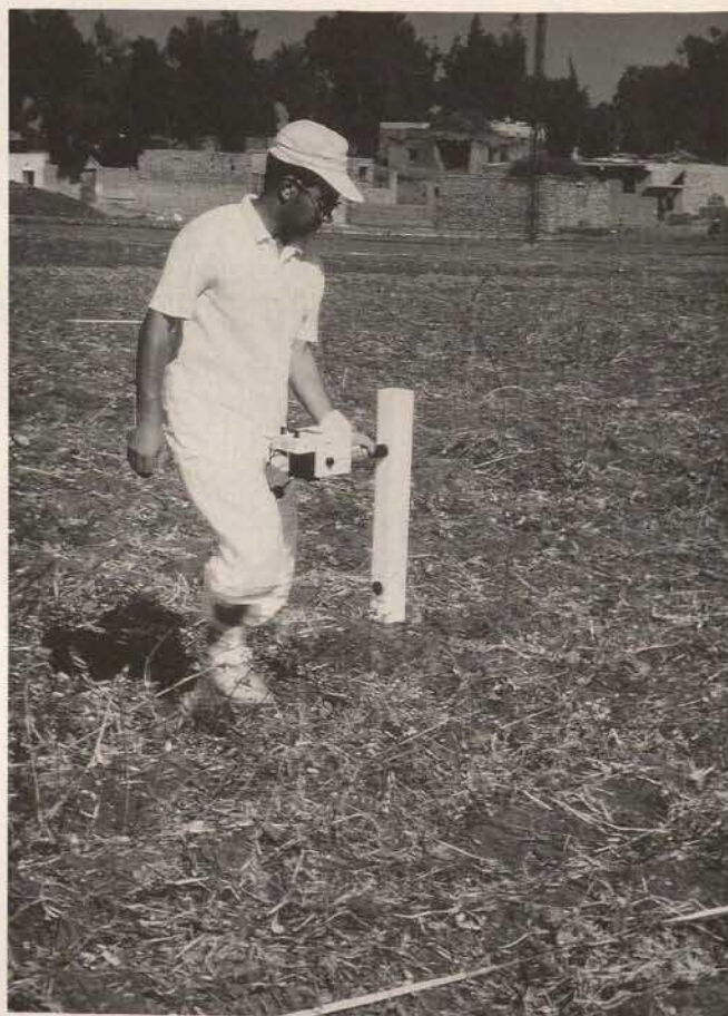
Fig. 1. Fluxgate Gradiometer Geoscan FM36 with distance trigger run by Tariq Fahmy of NRIAG National Research Institute for Astronomy and Geophysics, Helwan-Cairo (Photo by J. Fassbinder)
